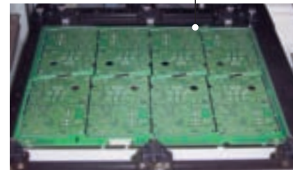
This is an image of a PCB inside the work board holder of the XY. Zierick's Model 9700 XY Terminal Insertion System is fully automatic, with a machine cycle rate of over 5,000 pph.
