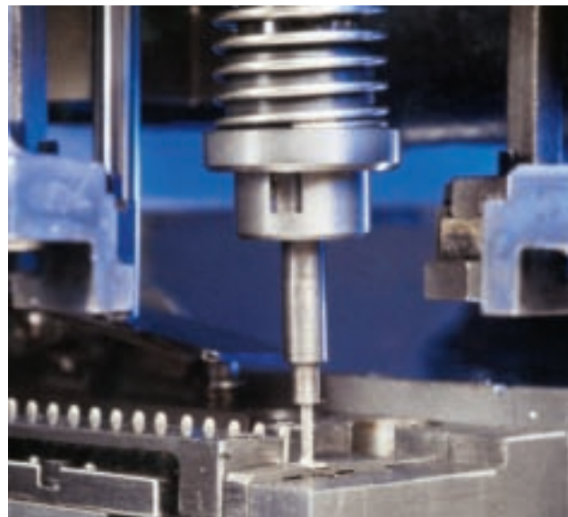
Surface Mount connectors are provided on a continuous reel of parts in strip form and are separated and presented to a vacuum pick-up nozzle by the feeder. Continuous Reels are supplied for Zierick SMT connectors such as Pins, Posts, IDCs, Tabs, Jumpers, Wire Grippers, Box Receptacles, and Clips.
