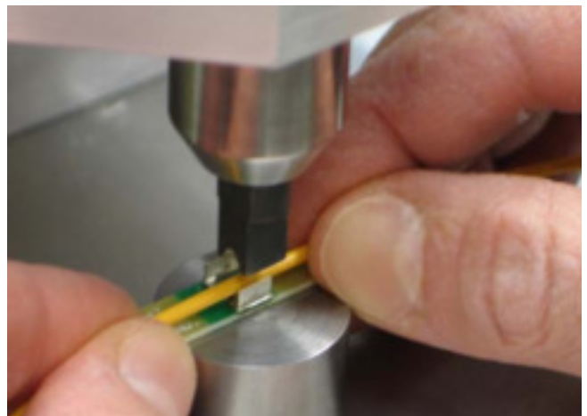
Figure 9. Wire in place for Insertion
