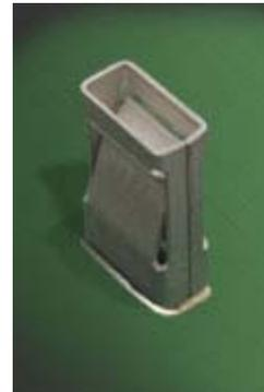
Manufactured for durability and reliability, the 1266 SMT Dual Entry Receptacle accommodates a minimum of twelve mating cycles without degradation. A higher mating cycle version is available. High locational tolerance results in geographic stability and a high pressure contact area accounts for a reliable gas tight connection.
