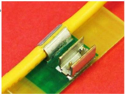
Zierick's wire-to-PCB connector solution combines the advantages of crimping, insulation piercing, and Surface Mount Technology into a highly reliable and economical way to terminate wires. If you'd like to read Zierick's winning Higgins-Caditz Award entry paper (.pdf), complete with all the engineering specs, usage, and test data, please click here.
